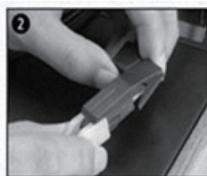
Take off and remove the stylus needle from the cartridge then replace with a new one
