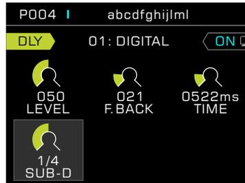
Press the TAP footswitch twice to control the delay time.
