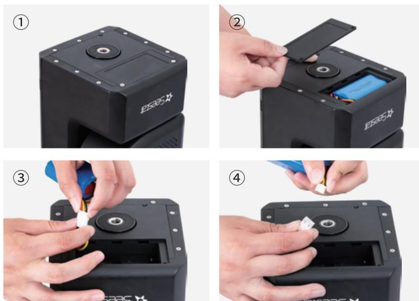
1. Note: Before replacing or removing the battery, make sure the device is turned off and disconnected from the power source. Additionally, handle the process with care to avoid damaging the device or battery.
