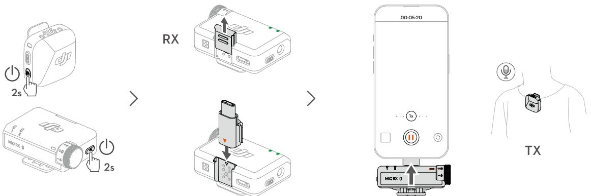
Press and hold the power button to power on the TX and RX. Mount the RX to the camera cold shoe, connect the audio cable, and then use the TX for audio recording.
