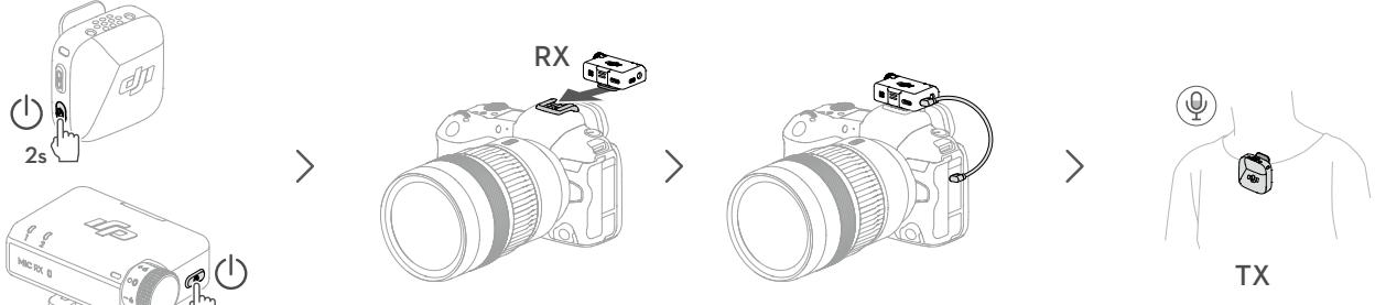
The TX can be used with Osmo Pocket 3 or Osmo Action 5 Pro. Select Wireless Microphone in the system settings and follow the on-screen instructions to complete the pairing.
