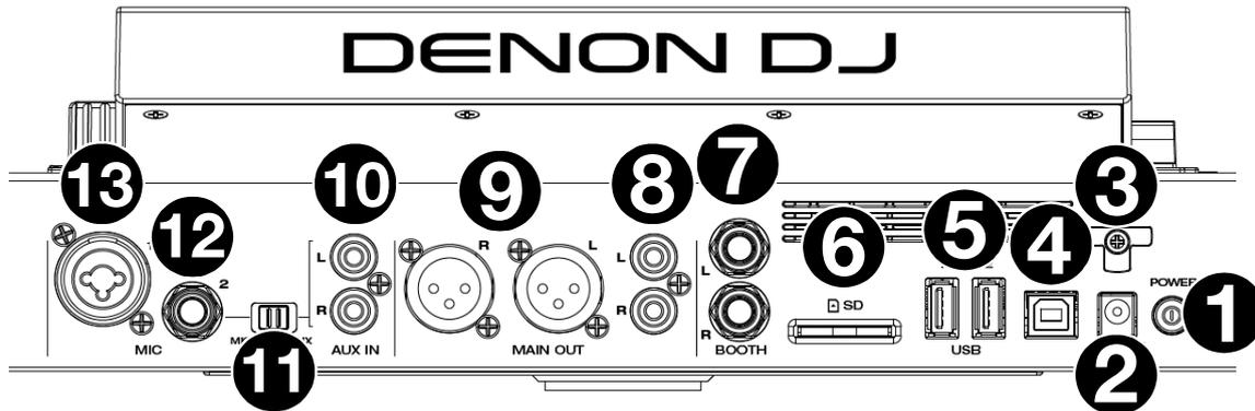
1. **Power Button:** Press this button to power SC LIVE 4 on. Power on SC LIVE 4 only **after** you have connected all your input devices and **before** you power on your amplifiers and loudspeakers.
