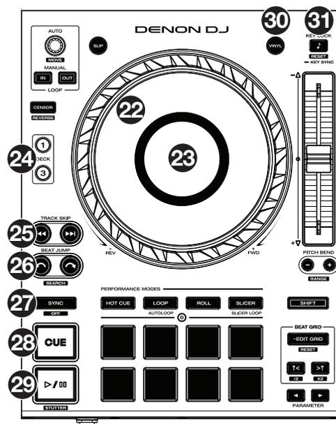
32. **Pitch Fader:** Move this fader to adjust the speed (pitch) of the track. You can adjust its total range with the **Pitch Bend** buttons.
