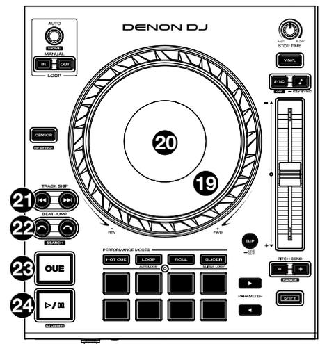
25. **Stop Time:** Controls the rate at which the track slows to a complete stop ("brake time") when you pause it by pressing **Play/Pause**.
