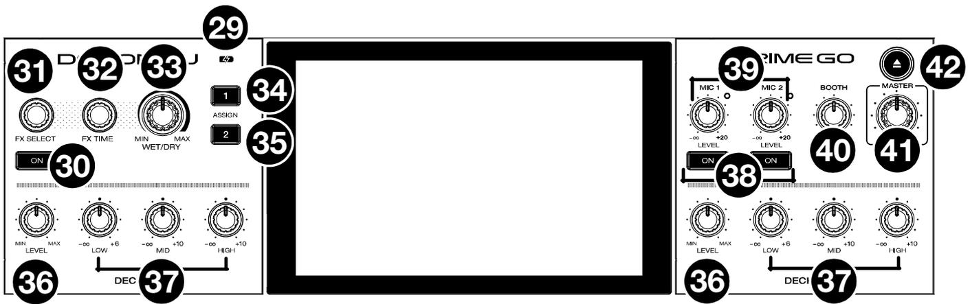
29. **Battery Charging Indicator:** This LED is solid green while charging. When charging is complete, the LED will turn off.
