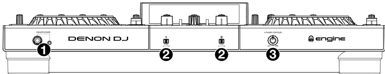
1. **Headphones (1/4", 1/8") (6.35 mm, 3.5 mm):** Connect your 1/4" or 1/8" (6.35 mm or 3.5 mm) headphones to this output for cueing and mix monitoring. The headphone volume is controlled using the **Phones Level** knob.
