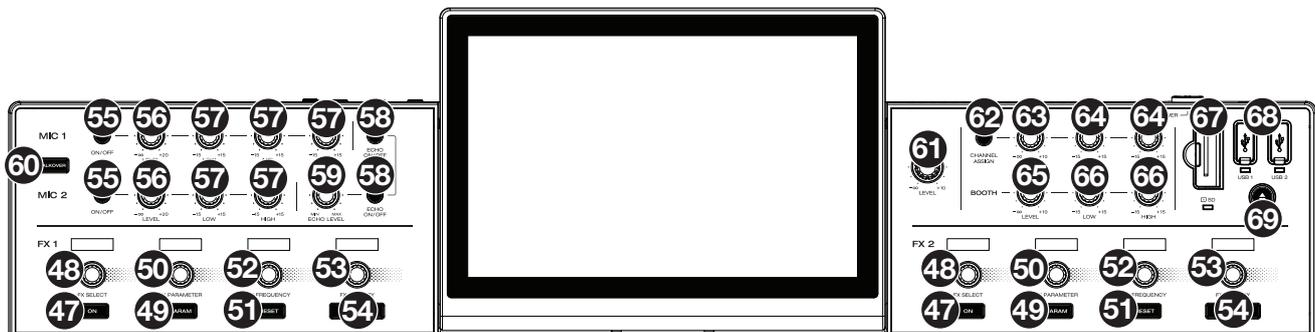
47. **FX On:** Press these buttons to enable or disable FX 1 and FX 2.
