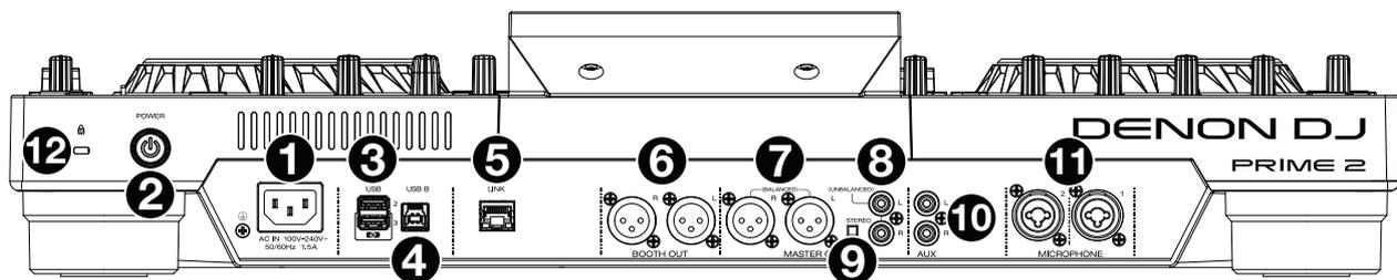
1. **Power Input:** Use the included power cable to connect this input to a power outlet. PRIME 2 has a protection circuit to safely eject all media after an unexpected power loss to protect your data from corruption. Reconnect your power source to return to normal operation.
