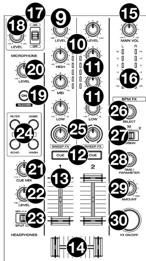
20. **Microphone Level:** Turn this knob to adjust the volume level for the microphone input. The **Peak** light next to the knob indicates the current signal level by its color: **green** (low), **amber** (normal/optimal), or **red** (maximum/peak). You can adjust additional microphone settings in the **Settings** menu.
