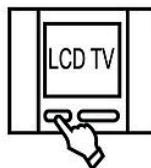
Hold down the "SET" button for about 6 seconds until the LED lights up. Then press the "VOLUME +" button. Check that the volume symbol appears on the TV. If it appears, press the SET button.
