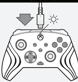
**EN** Plug the USB-C end of the cable into the top of the controller, and the USB side into your console or PC. The light above the Xbox logo will appear to indicate it is connected.
