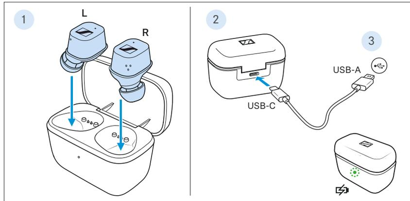
1. Open the charging case by overcoming a slight magnetic resistance and insert the left earbud into the left charging compartment and the right earbud into the right charging compartment. The earbuds are magnetically pulled into the charging compartments.
