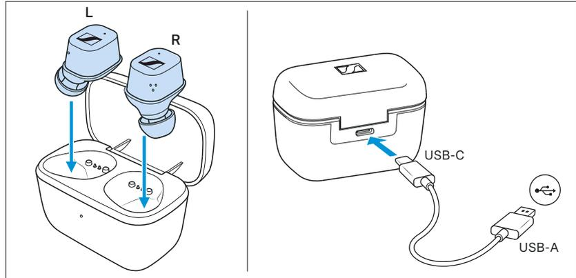
Upon delivery, the rechargeable batteries of the earbuds and the charging case are in sleep mode and have to be woken up by connecting them to a power source once.
