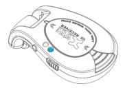
After connecting successfully, LED lights on receiver will keep light on.
