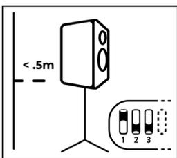
The speaker is on a monitor stand, and is within .5 meters (20 inches) of a wall, without being butted right against one.
