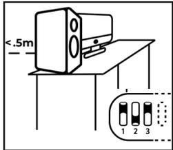
The speaker is on a desk or table, and is within .5 meters (20 inches) of a wall, without being butted right against one.
