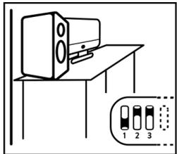
The speaker is on a desk or table, and is as close to a wall as possible without pinching any cables.
