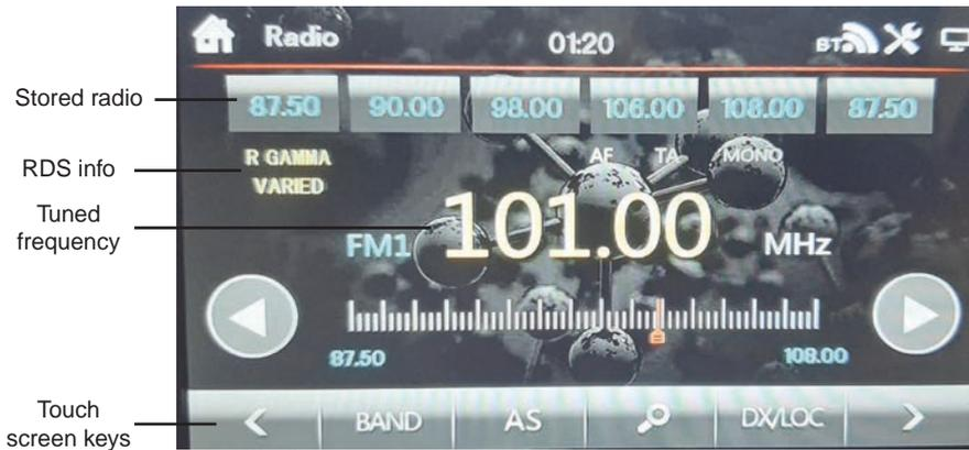
For the controls it is possible to use the touch screen directly (scroll the key bar to the right and left to see further function keys).
