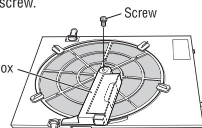
If the dust box unit is not attached properly, the inlet panel cannot be attached. Also, an abnormal (clattering) sound may be heard.
