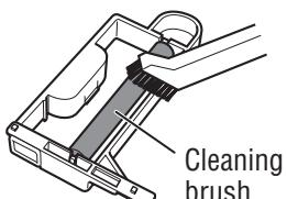
When the cleaning brush is very dirty, wash it in water, and then allow it to dry sufficiently.
