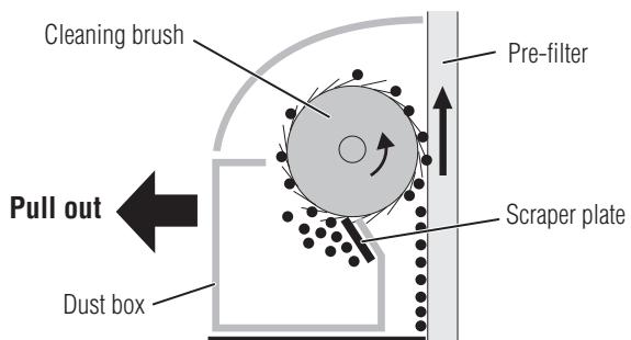
The dust accumulated on the scraper plate may gather together into a long belt-like shape that does not drop into the dust box. If the dust on the pre-filter is removed, the cleaning mechanism is working properly.
