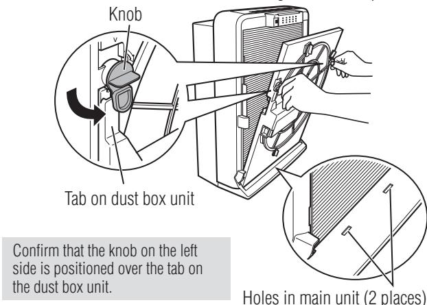
Confirm that the knob on the left side is positioned over the tab on the dust box unit.
