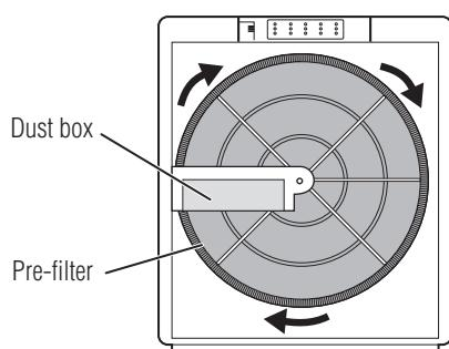
The dirt on the pre-filter is collected with the cleaning brush and accumulates on the scraper plate.
