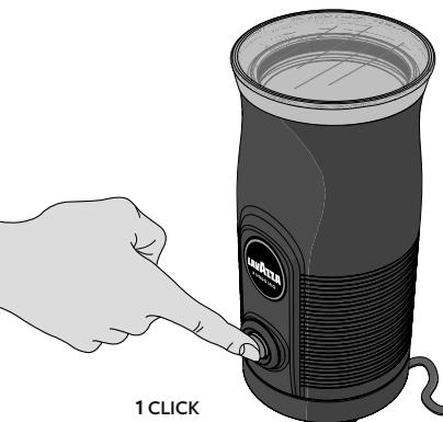
**⚠** Do not remove the milk frother from the base before completing the cycle.
