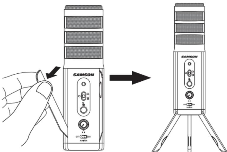
2. Set the Satellite's pattern switch. If you are recording a single person, set the switch to the Cardioid position and be sure to face the front side, with the Samson logo. If recording two people, set the microphone to the Bidirectional position and if recording multiple subjects, set the switch to the Omnidirectional position.
